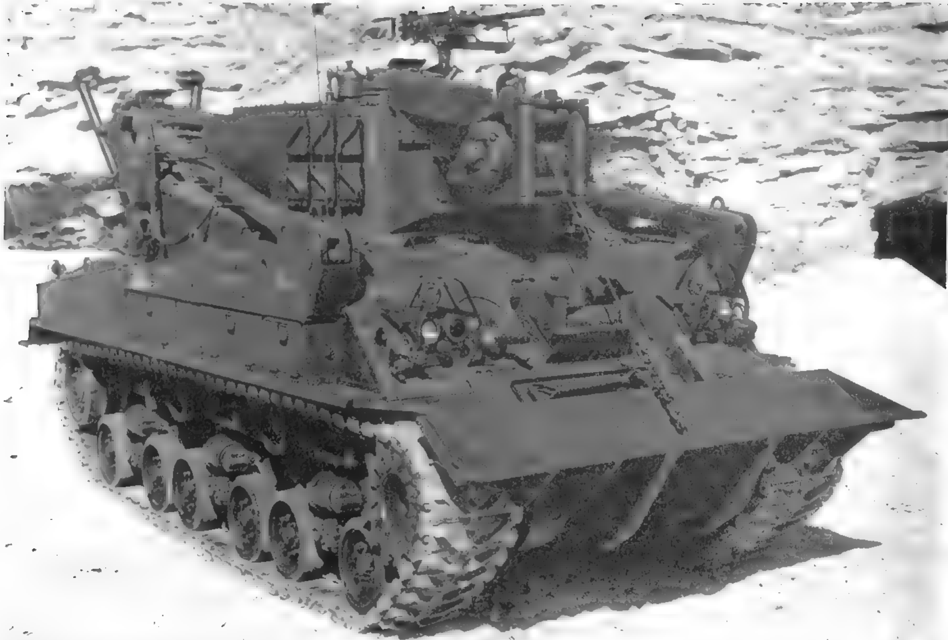
This M74 may well be the first one. Close examination of the stenciling discloses an October, 1953 date. Bowen-McLaughlin-York finished the first one in July 1953, and mass conversion of M4A3s into M74s did not begin until February 1954. In any event, it is factory fresh, as is evidenced by the scratch-free paint on the dozer blade. (Photo courtesy of the Patton Museum)
